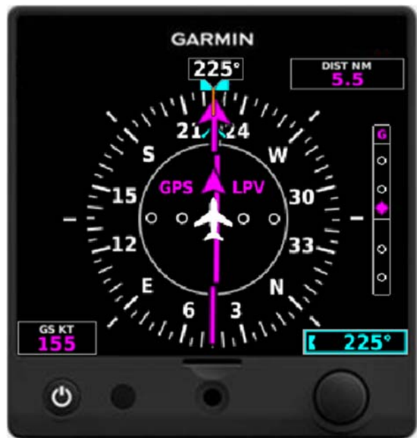
G5 Electronic Flight Instrument (HSI)
