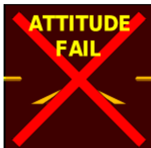
Attitude Failure Indication
