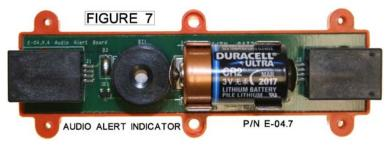
PLUG THE AUDIO ALERT CABLE P/N E-04.10.3 INTO THE RCPI UNIT, AND ONE END OF THE AUDIO ALERT INDICATOR. PLUG THE MALE END OF THE REMOTE CABLE P/N E-04.10.5 IN TO THE OTHER END OF THE AUDIO ALERT UNIT (FIG 8). MOUNT THE AUDIO ALERT UNIT BEHIND THE PANEL USING THE TWO CENTER SCREW ATTACH POINTS, AND 4-40 SCREWS, OR WITH INDUSTRIAL GRADE VELCRO ON THE BACK OF THE AUDIO ALERT (McMASTER CARR 94985K811) OR EQUIVALENT.
