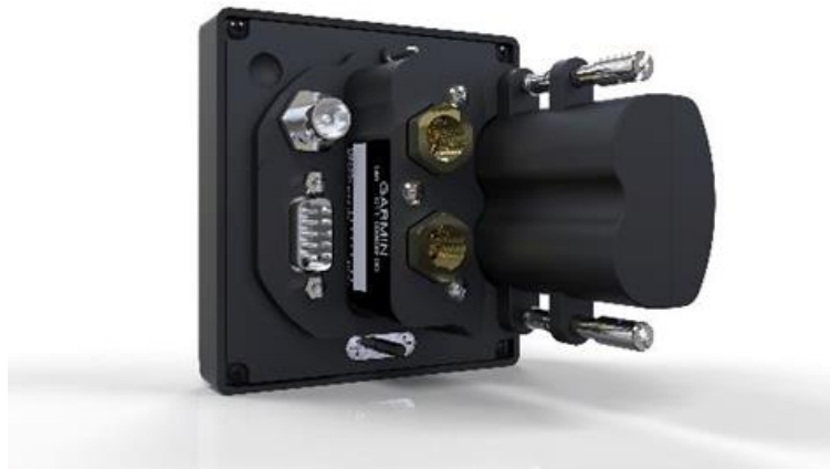
Figure 1-2 G5 Standby Battery
