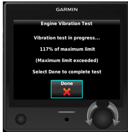
Figure 6-3 Engine Vibration Test Failure Indication
