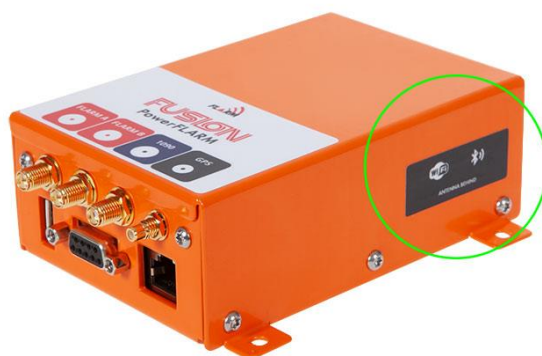
Wi-Fi and Bluetooth antenna location
