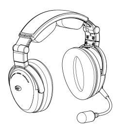
C. Position the microphone 1/8 inch from your mouth. Speak into the microphone side labeled "talk" which is marked at the microphone base.
